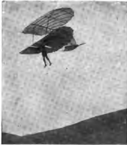
LILIENTHAL IN FREE FLIGHT ON HIS BIPLANE APPARATUS, SHOWING THE CHARACTER OF THE FRAMEWORK AND SHAPE OF THE PLANES, AS WELL AS THE REAR TAIL PIECE
